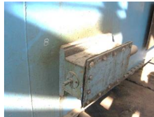
Redlers and transportation systems between the Extractor and the Toaster
