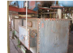
Redlers and transportation systems between the Extractor and the Toaster
